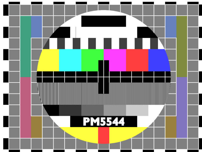
Figure 1a PM5544 test card properly displayed on a 110 degrees CRT using East-West correction
